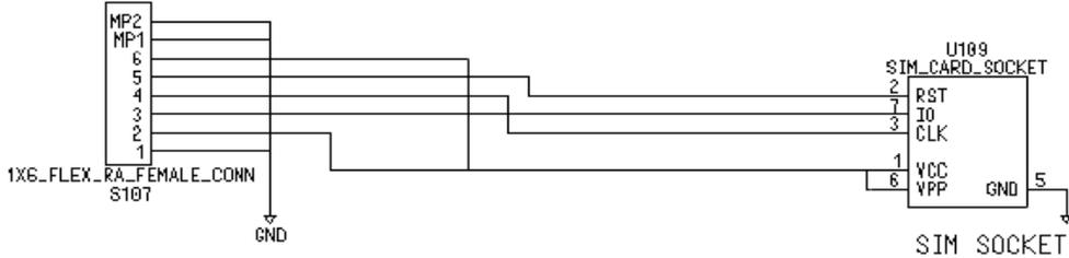
SIM Interface and Test Board integration
