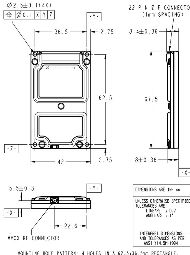
**Mechanical diagram of GPRS OEM radio modem**
