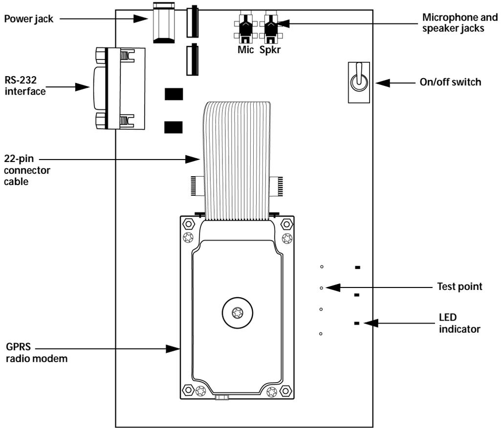
Interface and Test Board for on-board configuration – top view
